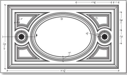
Reflected ceiling plan shows overall design and complete dimensions
