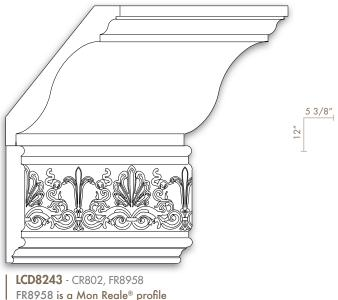
CR802 is a deeply profiled traditional crown moulding. It's large scale offers beautiful design variations. For additional height, and a richly finished detail, add the PM598, which has been designed specifically to fit the CR802.
