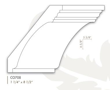
CO708 is a deeply profiled cove moulding and it's large scale offers beautiful design variations. For additional height, and a richly finished detail, add PM598, which has been designed specifically to fit CO708.
